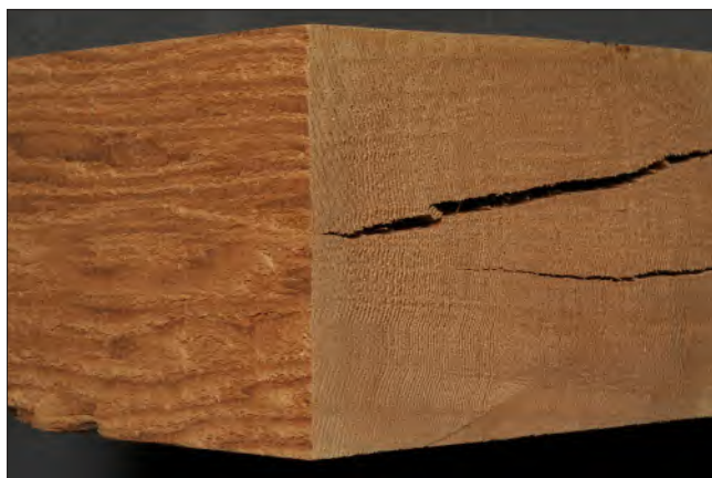
Figure 13-11. Red cedar timber end shows honeycomb (top). Surface of the timber shows no honeycomb (bottom).
